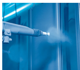
Coating treatment of external surface
