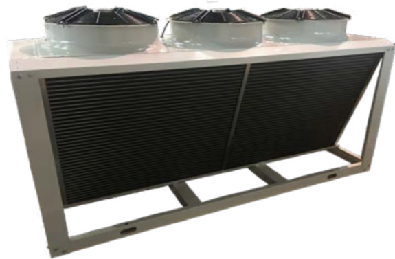
630mm V-type Condenser Number of fans: 1 ~ 3 Nominal Capacity: 28.2~110.9 kW
