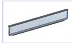
Insulating glass with metal edge sealing
